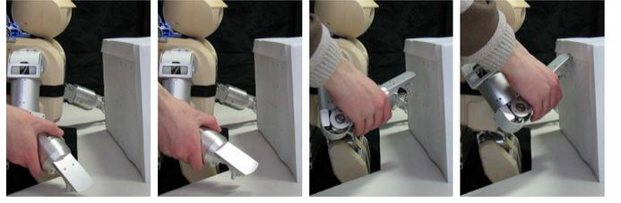
Fig. 3. Image sequence showing the teaching of the trajectories to HOAP-3 robot with kinesthetic demonstration. Teaching of reaching movements to CB-i was done in the same way.
