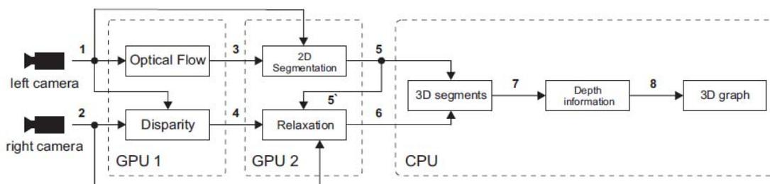
Fig. 1) Flow diagram of step 1: Extraction of 3D-graphs
