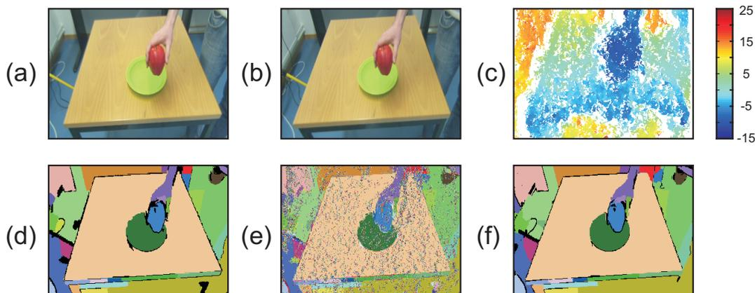
Figure 3. Segmentation of a stereo pair. (a) Original left frame  $\{t_L\}$ . (b) Original right frame  $\{t_R\}$ . (c) Estimated disparity map from phase-based stereo. (d) Extracted segments  $S_L^t$  for frame  $\{t_L\}$ . (e) Initialization of frame  $\{t_R\}$  after the spin transfer. (f) Extracted segments  $S_R^t$  for frame  $\{t_R\}$ .
