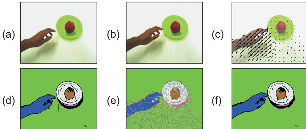
Figure 2. Segmentation of two adjacent frames in a sequence. (a) Original frame  $\{t\}$ . (b) Original frame  $\{t+1\}$ . (c) Estimated optical flow field from phase-based method (subsampling 16 times and scaled 5 times). (d) Extracted segments  $S_t$  for frame  $\{t\}$ . (e) Initialization of frame  $\{t+1\}$  after the spin transfer. (f) Extracted segments  $S_{t+1}$  for frame  $\{t+1\}$ .
