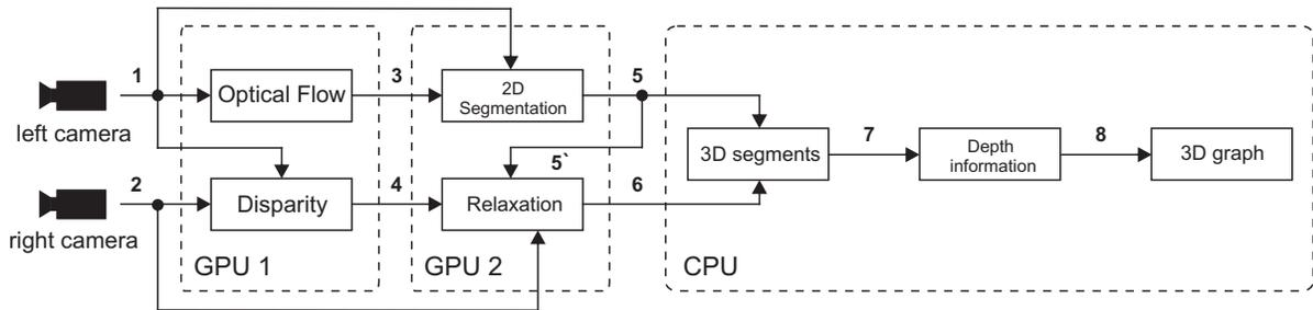
Figure 1. The architecture of 3D segment tracking framework.
