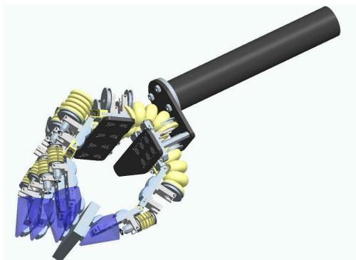
Fig. 3: Precise Three jaw grasp of the robotic hand
