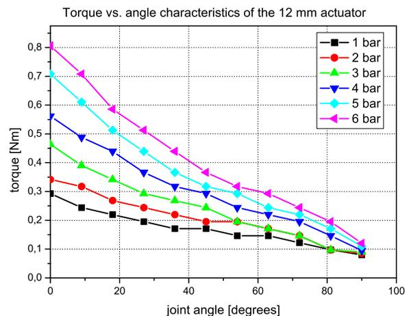
Fig 5: Torque vs. Angle plot for a 12 mm actuator
