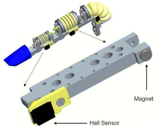
Fig. 9: Integration of the parts of the position encoder in a joint
