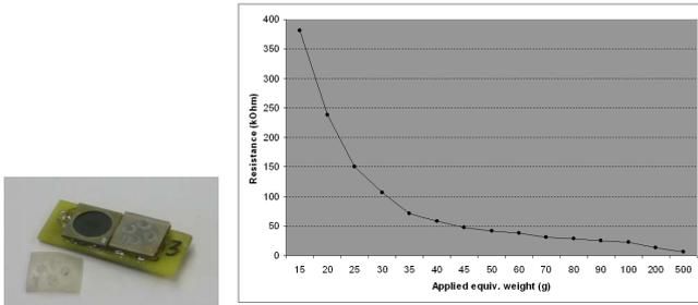
(a) Sensor array PCB with rubber actuation layer. (b) Characteristics of a subsensor
