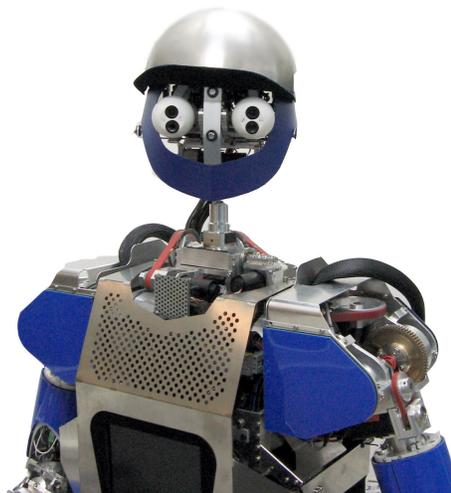
Fig. 1: The Karlsruhe humanoid head as part of the humanoid robot ARMAR-III. The head has two eyes and six microphones. Each eye has two camera
