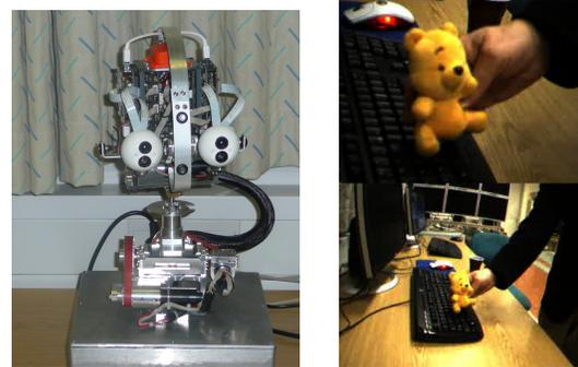
**Figure 1.** An example humanoid head (left). The narrow-angle cameras are positioned above the wide-angle ones. On the right are the images simultaneously taken from the wide- and narrow-angle view.
