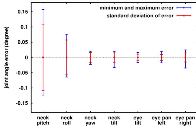
Figure 1: Accuracy of joint position during the repeatability tests. Each joint of the head was moved to the zero position starting from non-zero configurations 100 times. The pose of the head was measured visually using a calibration rig. The position error of the joints was measured using computer vision methods. The plot illustrates standard deviation, minimum and maximum of the joint angle errors in degrees.
