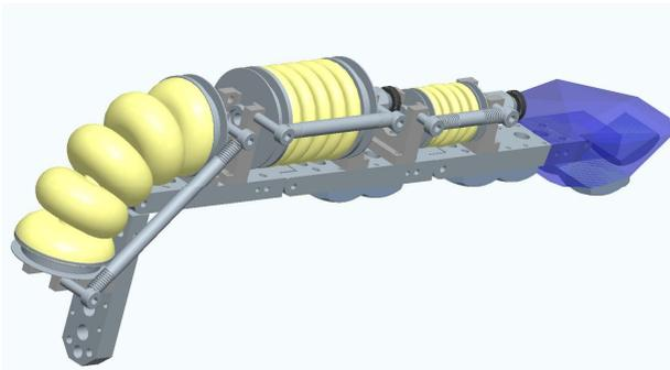
Fig. 7: Side view of a finger including actuation and retraction unit
