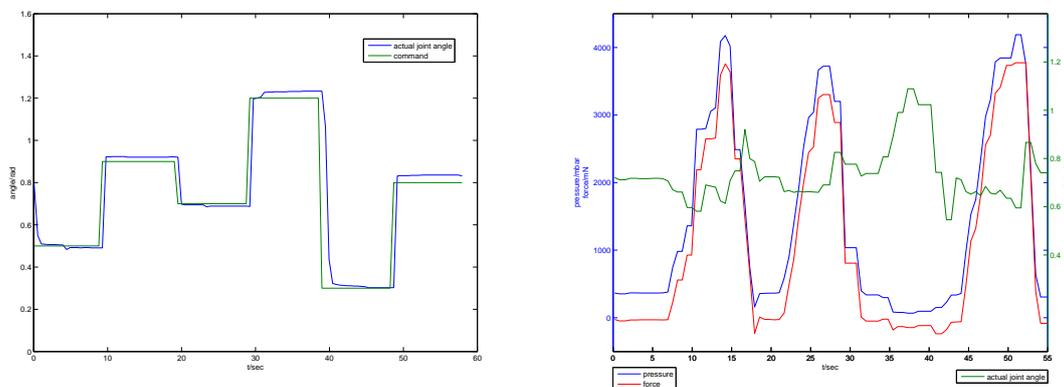
Figure 6: Response characteristics of a joint angle step command sequence for the index proximal joint (left) and typical response to external disturbances at a joint angle command of 0.7 rad and maximum force command (right). The three peaks in the pressure signal correspond to disturbances applied via external force.
