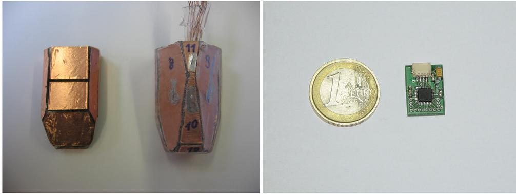
Figure 4: Finger tip with capacitive tactile sensor (left) and capacitive sensor electronics (right).
