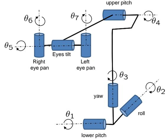
Fig. 2: The kinematics of the head with seven DoF arranged as lower pitch ( $\theta_1$ ), roll ( $\theta_2$ ), yaw ( $\theta_3$ ), upper pitch ( $\theta_4$ ), eyes tilt ( $\theta_5$ ), right eye pan ( $\theta_6$ ) and left eye pan ( $\theta_7$ ).
