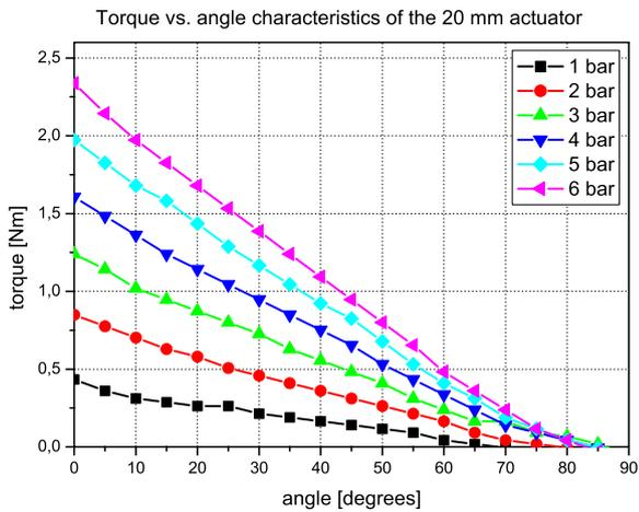
Fig. 6: Torque vs. Angle plot for a 20 mm actuator
