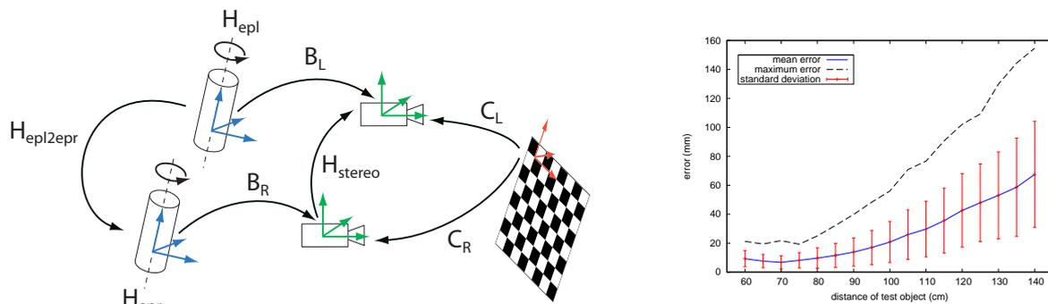
(a) Transformations involved in the kinematic calibration process for active stereo calibration. The aim was to find the unknown transformation  $B_L, B_R$  in order to derive  $H_{stereo}$  for actuated eyes.
