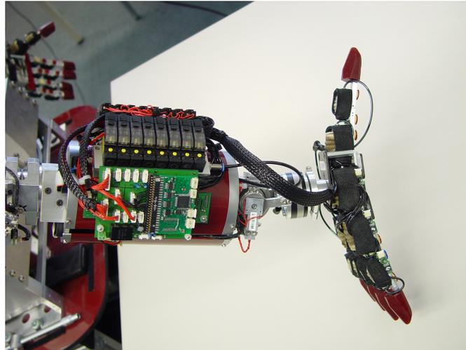
Figure 5: Pneumatic robot hand with sensors, valves and control system.
