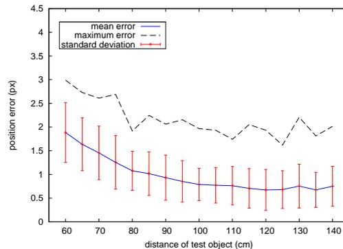
Figure 3: Accuracy of a saccadic eye movement tasks. The target object was positioned at arbitrary locations and different distances. The error is given in pixels.
