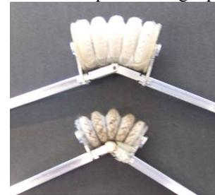
Fig. 4: Flexible fluidic actuators 20 mm (top), 12 mm (bottom)
