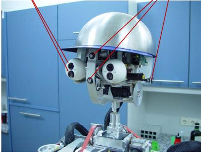
Fig. 3: The humanoid head with seven DoF arranged as lower pitch, roll, yaw, upper pitch, eyes tilt, left eye pan and right eye pan.
