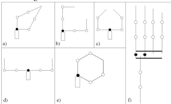
Fig. 2: Schematic sketches of the realizable grip patterns (a-e) and basic outline of the hand structure (f).
