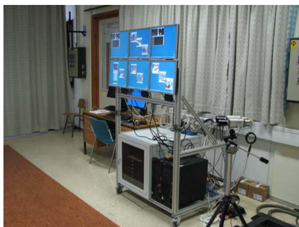
Fig. 4: Computer Cluster at JSI: six servers, two workstations, 1 Gbit Ethernet networks
