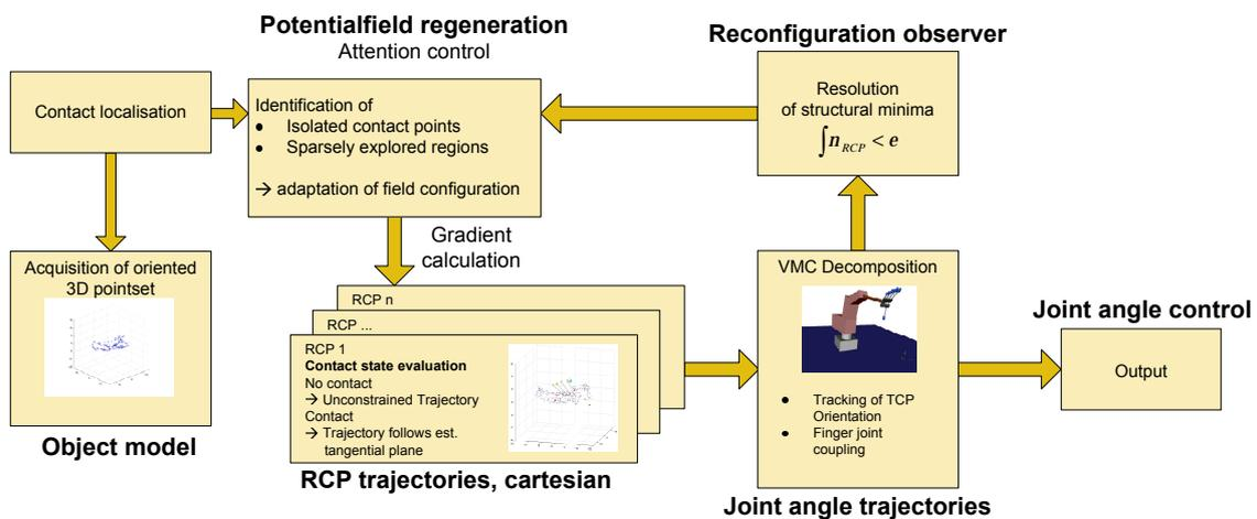
Figure 4: Tactile exploration scheme based on dynamic potential field.
