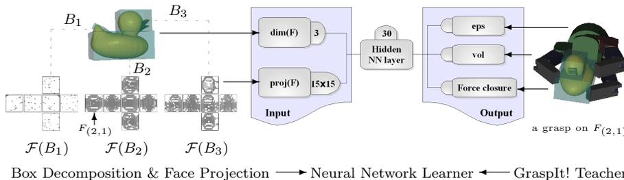
Figure 12: The applied neural network structure holds 228 input, 30 hidden and 3 output neurons. As an input, a face projection  $F$  plus its box dimensions  $dim(F)$  are fed into the network, since faces are normalized to  $15 \times 15$ .  $eps$  and  $vol$  are the grasp quality measures that GraspIt! delivers. The force closure is also learned separately even if it equals ( $eps > 0$ ). From this model, off-line learning of grasp qualities from face representations is made available.
