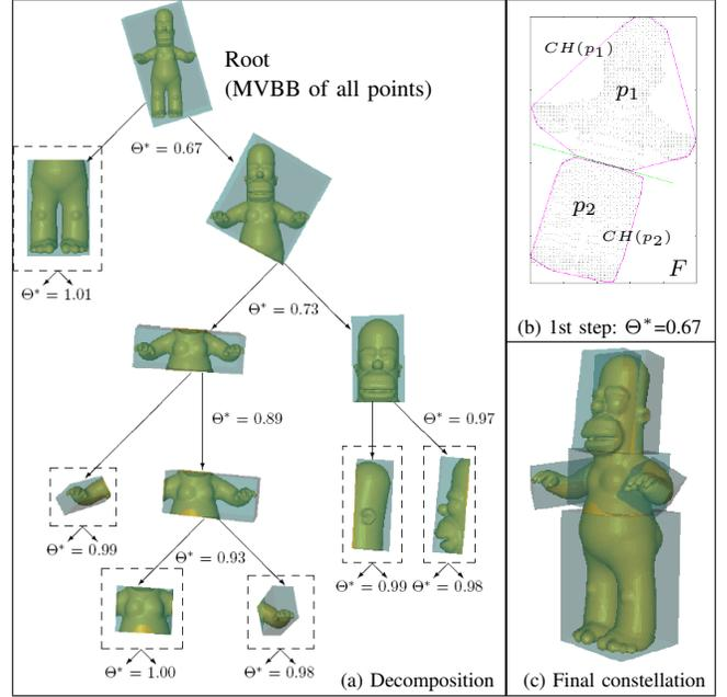
Fig. 2. (a) Example of a decomposition hierarchy, using a gain parameter of  $t=0.98$ . With  $\Theta^* < t$ , a valid cut is detected, as presented for the first step in (b). Otherwise, the box is a leaf box (dashed), i.e. a part of the final constellation which is plotted in (c).
