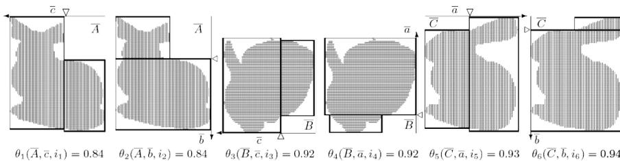
Figure 2: Best cuts along the six box directions and cut positions  $i$  (triangles). The corresponding volume values  $\theta(\bar{\mathcal{F}}, \bar{f}, i)$  (according to (1)) are also presented.
