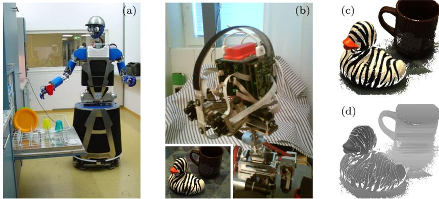
Figure 13: (a) The Armar-III humanoid platform (Asfour *et al.*, 2006) used in the PACO-PLUS project. (b) A duplicate of the Armar-III stereo head, used in our lab, including a clipped region of an acquired rectified image. (c) Result of image differencing related to an image without the objects. This mask is applied in (d) to results from the disparity processor. Note that apart from white being the mask region, intensity corresponds to distance to the viewpoint.
