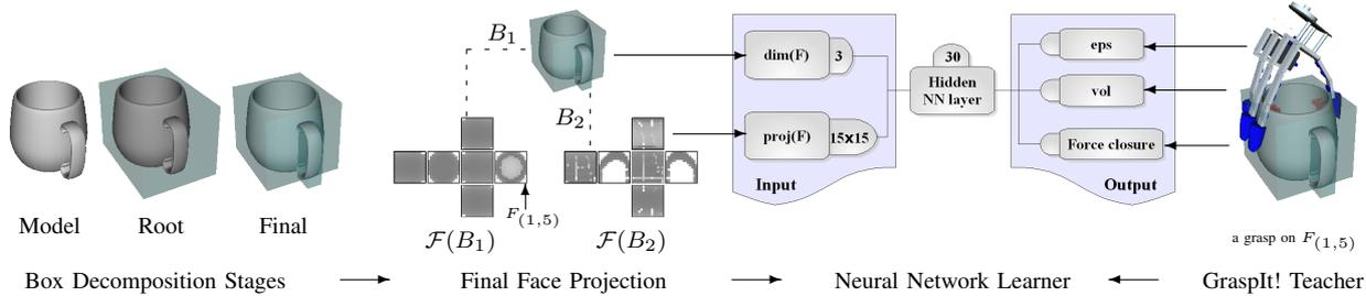
Fig. 3. The applied neural network structure holds 228 input, 30 hidden and 3 output neurons. As an input, a face projection  $F$  plus its box dimensions  $dim(F)$  are fed into the network, since faces are normalized to  $15 \times 15$ .  $eps$  and  $vol$  are the grasp quality measures that GraspIt! delivers. The force closure is also learned separately even if it equals ( $eps > 0$ ). From this model, off-line learning of grasp qualities from face representations is possible.
