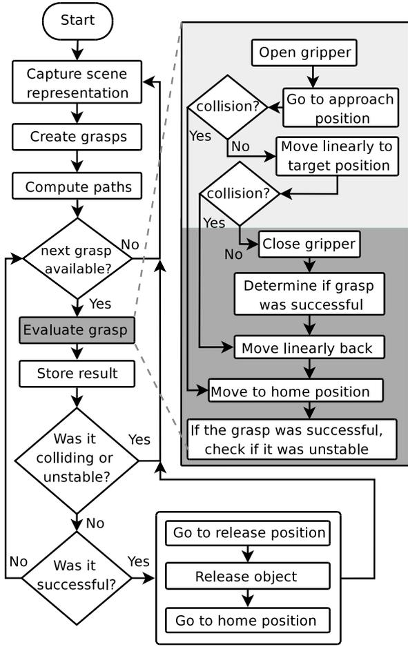
Fig. 5. Flow diagram for the process of creating and evaluating grasping hypotheses automatically. The bright part (top right) indicates the utilization of active collision detection.
