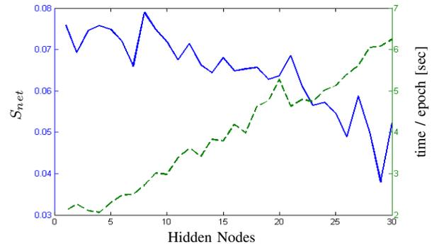
Fig. 7. Success (solid) and training time (dashed) for different number of hidden nodes with the leave-one-object-out validation, averaged over 10 runs. The maximum success value of  $S_{net} = 0.078$  was detected at 8 nodes.
