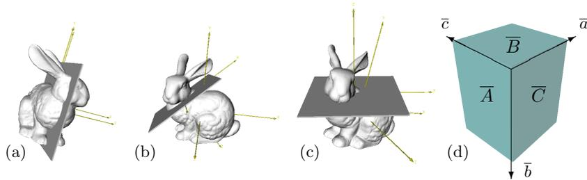
Figure 1: Exemplary cuts of the bunny: (a) a central cut, (b) an intuitively best cut and (c) a good cut parallel to one of the root MVBB planes. (d) Restriction to surface-parallel cutting planes in the simple approach.
