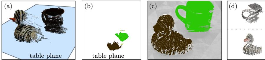
Figure 14: (a) Scene reconstructed from Fig. 13d, purged by table plane assumption. (b) Objects deduced from 2.5D segmentation on table plane projection. Note that the table is not detected, but just the (infinite) table plane visualized. (c) Reprojection of the segmented 3D objects (d) to the image.
