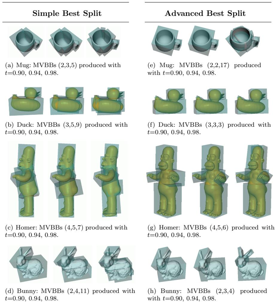
Figure 5: Examples of box decomposition using different gain thresholds  $t=0.90, 0.94, 0.98$ , where numbers in brackets correspond to numbers of boxes. (a)-(d) show the results with the simple cutting proposed in Section 4.3, while (e)-(h) shows the advanced cutting proposed in Section 4.4.
