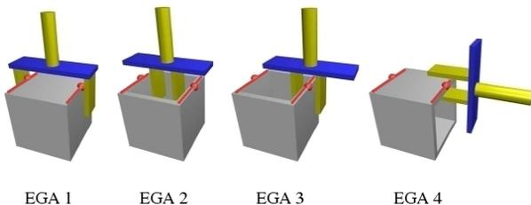
Fig. 3. Elementary grasping actions (EGAs). Red lines indicate 3D contours, red dots their center. EGA3 and EGA4 can each be defined with two different positions — one for each contour.
