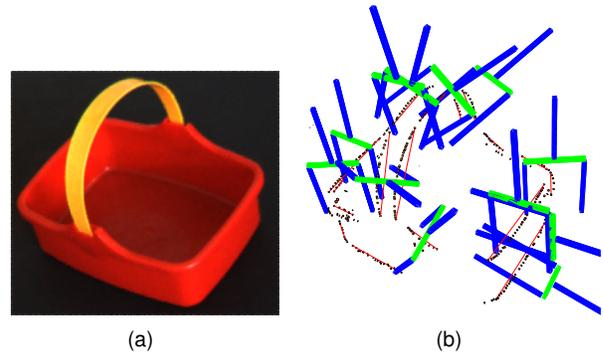
Fig. 4. Generation of multiple grasping hypotheses. (a) A sample object. (b) Grasping hypotheses generated for the sample object. Note that not all of them will lead to successful grasps.
