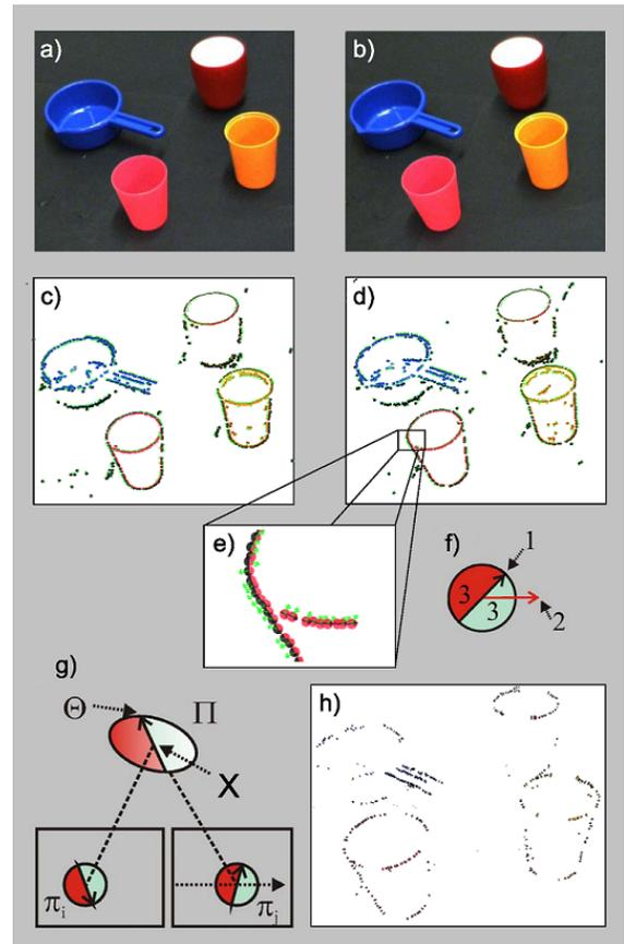
Fig. 2. The extraction of primitives. (a,b) show the original left and right image. (c,d) show the corresponding 2D primitives. (e,f) show a close up of the 2D primitives and their modalities: orientation (1), phase (2) and color (3). (g) illustrates the reconstruction of a 3D primitive using two 2D primitives. (h) shows the resulting 3D primitives.
