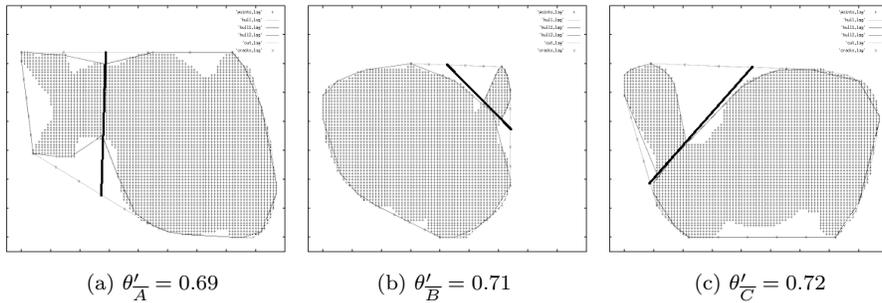
Figure 4: The three best projection splits when using the advanced convex hull algorithm. The result is much more confident than those derived from Fig. 1, while the additional computational effort is still acceptable.
