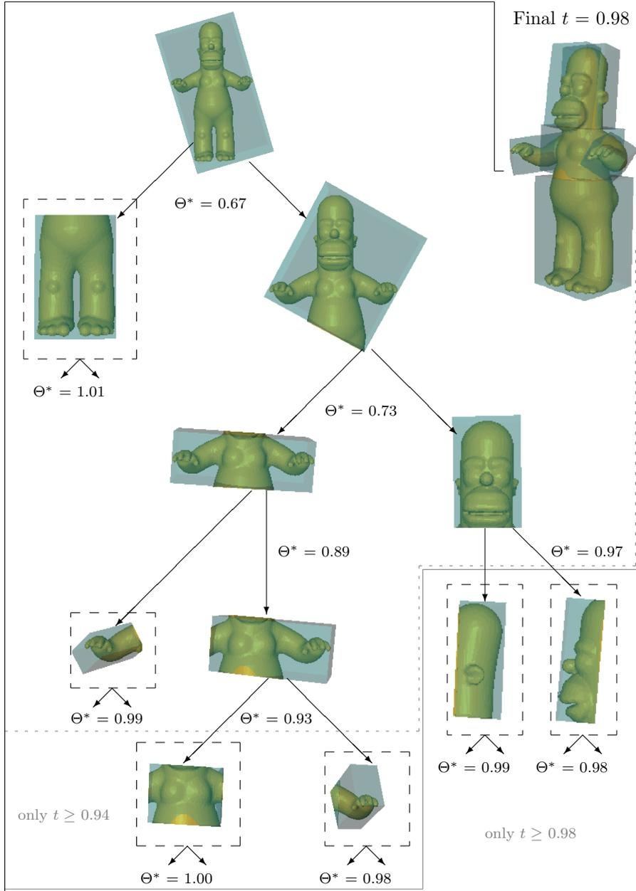
Figure 6: Visualization of a decomposition hierarchy. The example shows a model decomposition, using a gain threshold  $t = 0.98$ . Is the best volume split value  $\Theta^*$  below this threshold, a valid cut is detected. Otherwise, the box is a leaf box (*dashed*), a part of the final constellation. One can also trace the results with lower thresholds ( $t = 0.9$  dotted gray;  $t = 0.94$  solid gray) from Fig. 5g.
