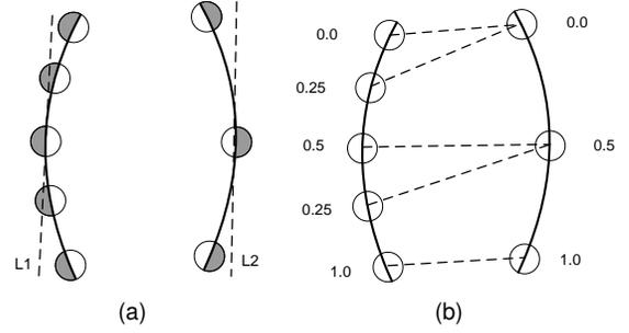
Fig. 6. (a) Whether the left or the right color of a contour is used for the co-linearity computation is determined by the contour's position relative to the line which is defined by the center and the first principal component vector of the other contour. (b) Dashed lines indicate the pairing of primitives, used for relations that do not address the entire contours.
