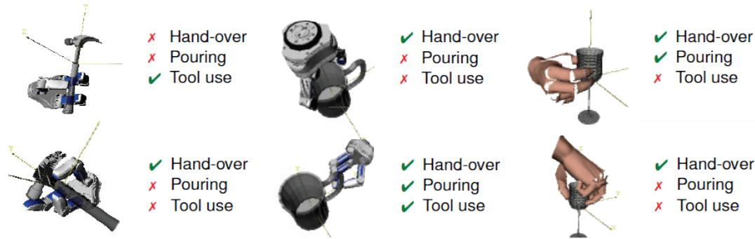
\* Grasps are automatically generated from box-based representations, the labels have been assigned manually.
