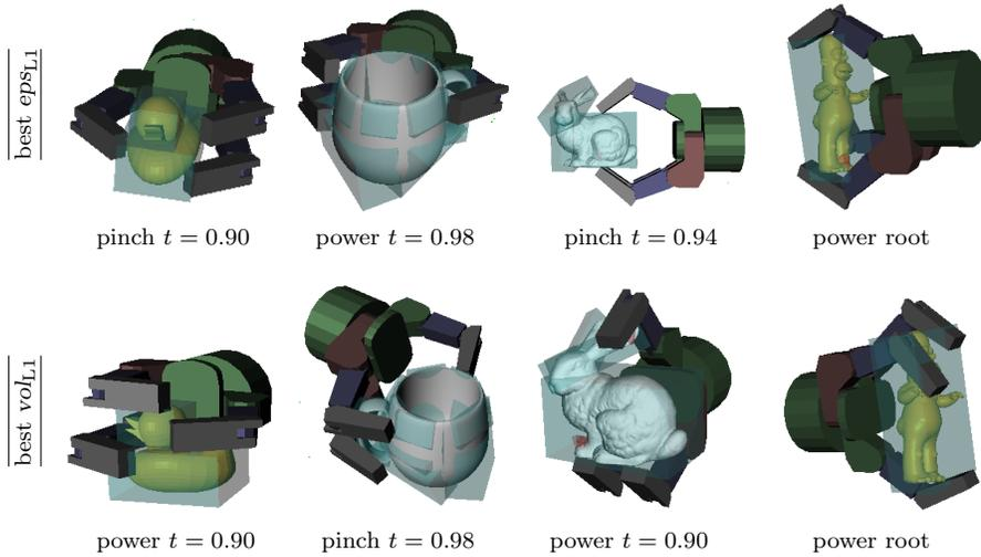
Figure 7: Best grasps for the experimental Barrett hand grasping results in Tab. 2. Upper row: best  $eps_{L1}$  grasps. Bottom row: best  $vol_{L1}$  grasps.
