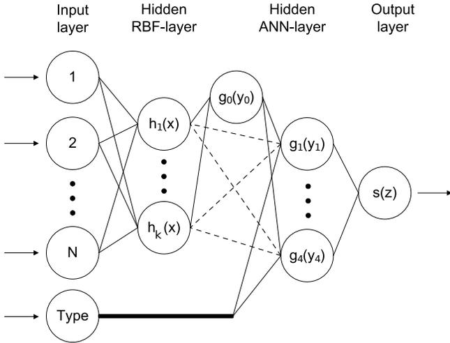
Fig. 7. Architecture of neural network. The input is given by an  $N$ -dimensional feature vector and the type of the corresponding hypothesis. The output reflects the likelihood for the grasping hypothesis to be successful. The 0'th neuron in the hidden ANN-layer provides a bias for the other four neurons. The dashed lines connecting them to the RBF-neurons represent the weights that are obtained during learning.
