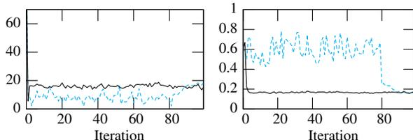
Fig. 8. Illustration of the effect of inverse kinematics sampling on the overall edge and distance error by the example of the person’s right arm shown in Fig. 6. The solid line indicates the result computed with inverse kinematics sampling, the dashed line without. Left: Euclidean distance error in [mm]. Right: edge error.
