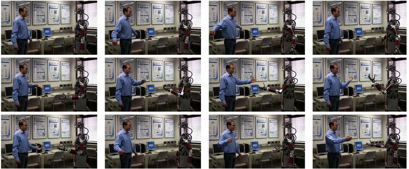
Fig. 7. Image samples of the online imitation of human motion by the humanoid ARMAR-IIIb.
