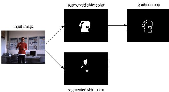
Fig. 3. Illustration of the image processing pipeline.
