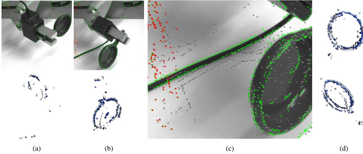
**Fig. 4.** Birth of an object (a)-(b) top:2D projection of the accumulated 3D representation and newly introduced primitives, bottom:accumulated 3D representation. (c) newly introduced and accumulated primitives in detailed. Note that, the primitives that are not updated are red and the ones that have low confidence are grey (d) final accumulated 3D representation from two different poses.
