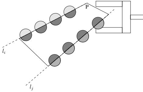
Fig. 4. A set of spatial primitives on two different contours  $l_i$  and  $l_j$  that have co-planarity, co-colority and collinearity relations; a plane  $P$  defined by the co-planarity of the spatial primitives and an example grasp suggested by the plane.
