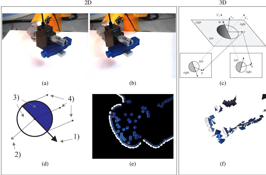
**Fig. 1.** Overview of the system. (a)-(b) images of the scene as viewed by the left and right camera at the first frame. (d) symbolic representation of a primitive: wherein 1) shows the orientation, 2) the phase, 3) the colour and 4) the optic flow of the primitive. (e) 2D-primitives of a detail of the object. (c) reconstruction of a 3D-primitive from a stereo-pair of 2D-primitives. (f) 3D-primitives reconstructed from the scene.
