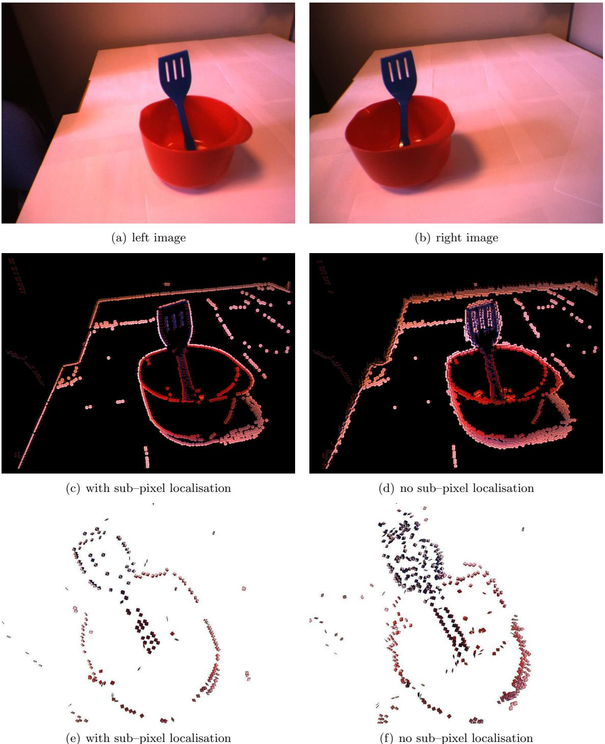
Figure 16: Reconstruction of 3D-primitives in a real scenario. The two stereo images are shown in (a) and (b) (resp. (c)) (resp. without) sub-pixel localisation; and (e) (resp. (f)): spatial primitives reconstructed with (resp. without) sub-pixel localisation.
