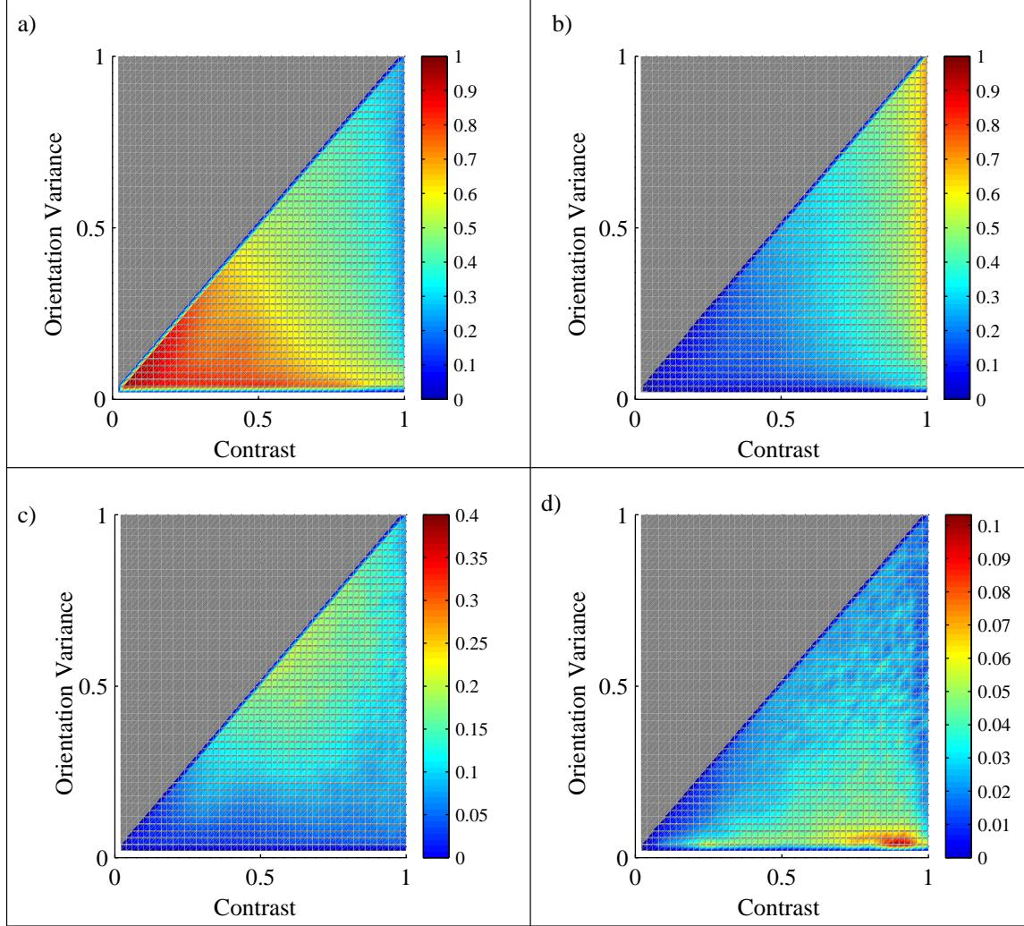
Figure 6.  $P(\text{3D Discontinuity} \mid \text{2D Structure})$ : (a)  $P(\text{Continuity} \mid \text{2D Structure})$ . (b)  $P(\text{Gap Discontinuity} \mid \text{2D Structure})$ . (c)  $P(\text{Irregular Gap Discontinuity} \mid \text{2D Structure})$ . (d)  $P(\text{Orientation Discontinuity} \mid \text{2D Structure})$ .
