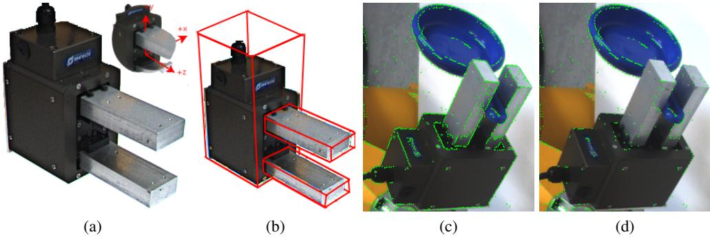
**Fig.3.** Gripper elimination (a) grasper and grasper coordinate system (b) bounding boxes of grasper body and its fingers (c) primitives before grasper elimination (d) primitives after grasper elimination
