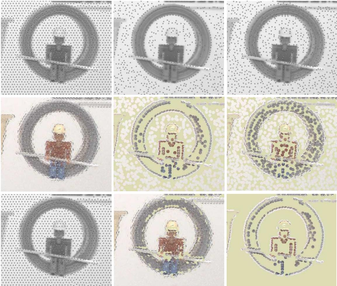
Figure 9: Top row: positions associated to the primitives assuming different intrinsic dimensionality (from left to right, i0D, i1D and i2D). Middle row: Primitives in each of those cases (from left to right, i0D, i1D and i2D). Bottom row, left: positions using the interpretation given by the intrinsic dimension with the highest confidence; middle: primitives extracted at those locations; and right: primitives at non-i0D locations.
