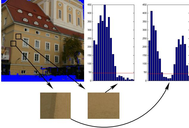
Figure 4. Example histograms and the number of clusters that the function  $\psi(S)$  computes.  $\psi(S)$  finds one cluster in the left histogram and two clusters in the right histogram. Red line marks the threshold value of the function. X axis denotes the values for 3D orientation differences.
