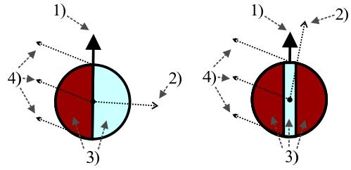
(a) An edge primitive    (b) A line primitive
