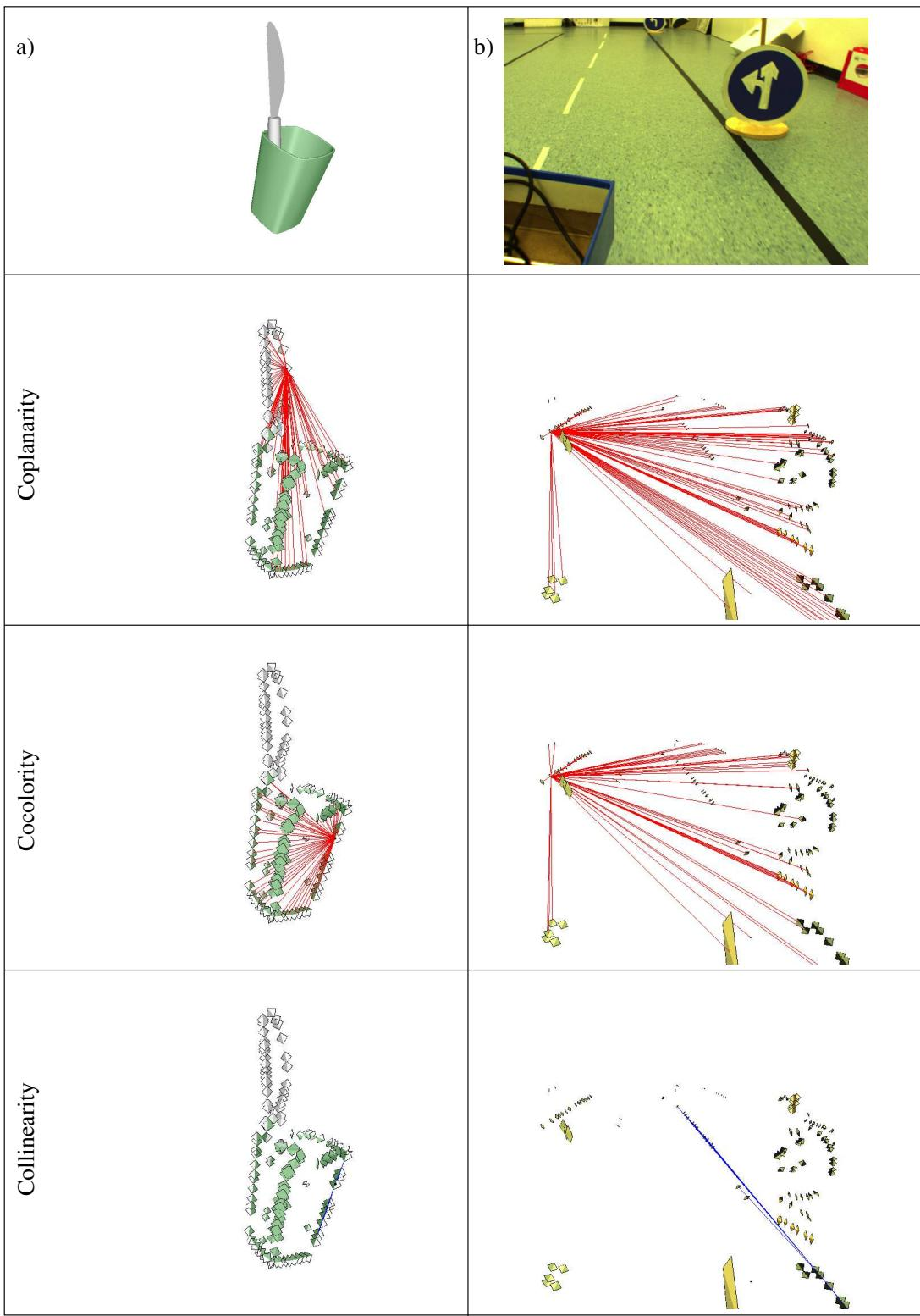
Figure 6: The coplanarity, cocolority and collinearity relations on two different examples shown in (a) and (b). The results are from our 3D display tool called *Wanderer*, and for the sake of speed, 3D primitives are shown in squares. The relations are shown only for a selected primitive as showing relations between all primitives disables visibility.
