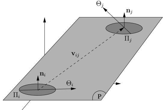
(a) Co-planarity of two 3D primitives  $\Pi_i$  and  $\Pi_j$ .
