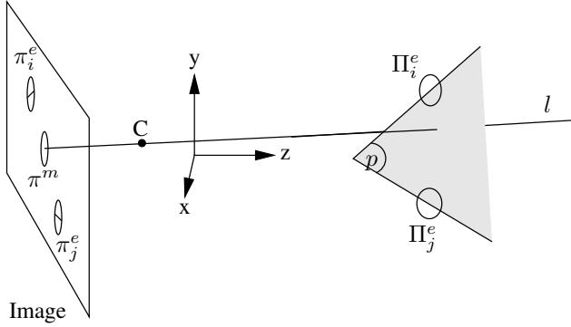
Figure 9: Illustration of how the vote of a pair of edge primitives is computed. The 3D primitives  $\Pi_i^e$  and  $\Pi_j^e$  corresponding to the 2D primitives  $\pi_i^e$  and  $\pi_j^e$  define the plane  $p$ . The intersection of  $p$  with the ray  $l$  that goes through the 2D mono  $\pi^m$  and the camera center  $C$  then determines the position of the estimated 3D mono  $\Pi^m$ . The 3D orientation of  $\Pi^m$  is set to be the orientation of the plane  $p$ .
